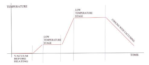
1)Before the silicone bag shelf being pushed into the oven, start the vacuum pump to vacuuming for 3-5 minutes. Check whether the silicone bag is leaking or not. And the vacuum value should at least be 0.095Mpa.
